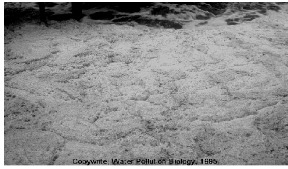
Nocardia Foam on the Surface of Aeration Basin
