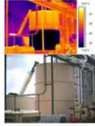
Liquid Storage tank Determination of liquid level.
