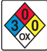
Sodium Hypochlorite NFPA Chemical Hazard Label
