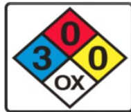
Sodium Hypochlorite NFPA Chemical Hazard Label
