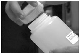
Before turning on the water to draw the sample, remove the cap from the container and position it under the faucet. Turn on the cold water tap and begin filling the container.
