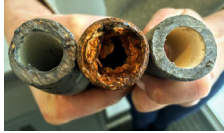
Orthophosphates bond to lead pipes
